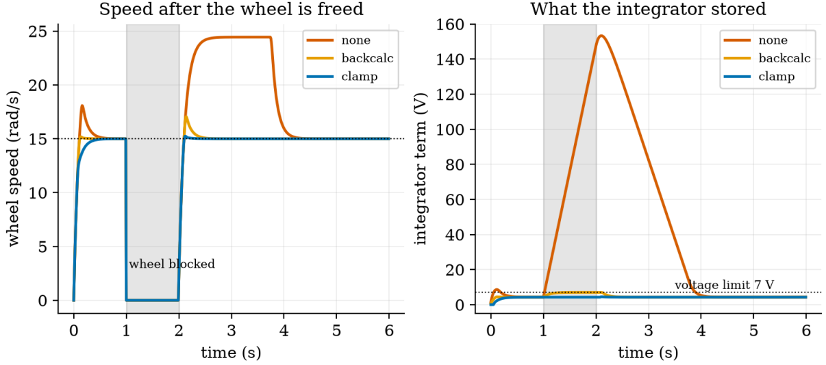
Left: wheel speed when the wheel is blocked from 1 s to 2 s with a setpoint of 15 rad/s: without anti-windup (red) it surges to 24.4 rad/s after release and recovers in 2.1 s; back-calculation (orange) peaks at 17.1 rad/s; clamping (blue) at 15.2 rad/s. Right: the integrator term: 146 V stored without protection against the 7 V the motor can use; 7.0 V and 4.3 V with the two methods.
